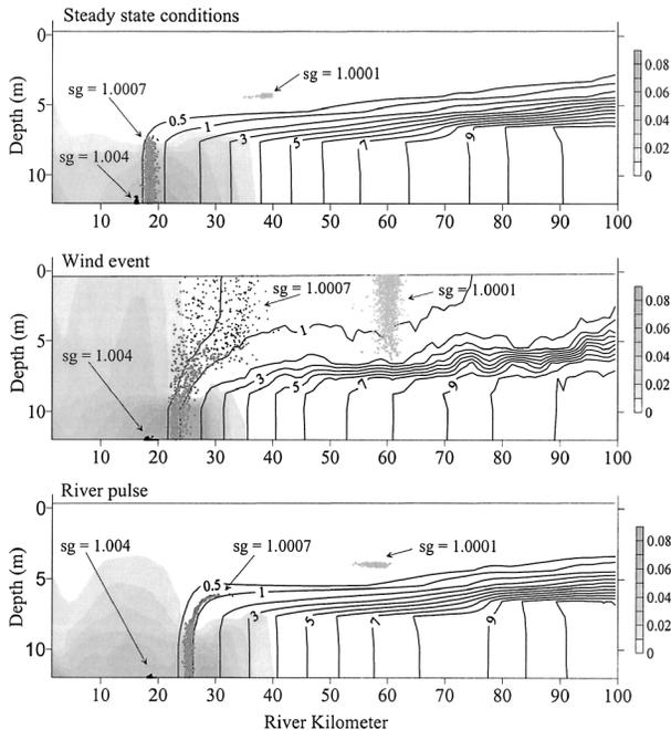
Fig. 9. Salinity (psu, line contours), suspended sediment concentrations ( $\text{kg m}^{-3}$ , shaded contours), and distribution of striped bass egg-like particles 2 d after release throughout the water column at river kilometer 16 in steady state, wind event, and river pulse conditions. The locations of 3 sets of egg-like particles are depicted in each panel, those with specific gravities (sg) of 1.0001 (light gray), 1.0007 (dark gray), and 1.004 (black).
