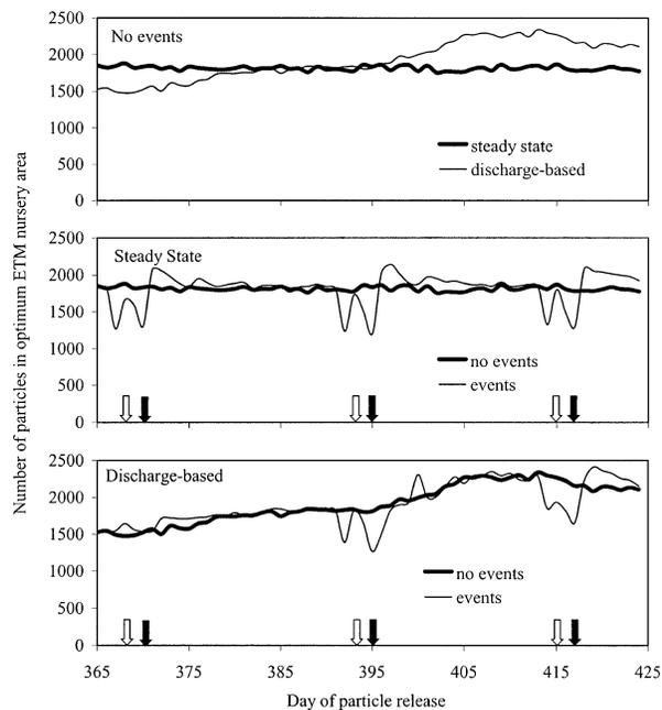
Fig. 11. Number of egg-like particles in optimum nursery area versus time (day on which particles were released) in steady-state and discharge-based scenarios with no episodic events, steady-state scenarios with and without wind and river pulse events, and discharge-based scenarios with and without wind and river pulse events. Arrows indicate the start time of 21-h wind (white arrow) and 2-d river pulse (black arrow) events.
