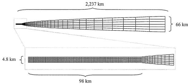
Fig. 4. Schematic of model domain. Upper diagram represents the entire model domain. Lower diagram illustrates the grid line geometry of the channel, the region of interest. Reproduced from North et al. 2004.
