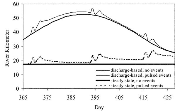
Fig. 10. Location of the salt front (intersection of the 0.5 psu isohaline with the bottom) over time for steady-state (lower lines) and discharge-based (upper lines) scenarios without wind events and river pulses (smooth lines) and with them (lines with small peaks).
