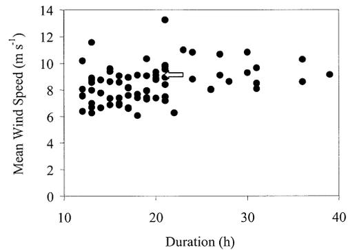
Fig. 1. Mean wind speed (m s<sup>-1</sup>) versus duration (h) of down-estuary wind events in April and May 1986–2002 in upper Chesapeake Bay measured at Thomas Point Light. The white arrow indicates the duration (21 h) and magnitude (9.1 m s<sup>-1</sup> wind speed) of down-estuary wind events used in numerical model scenarios.
