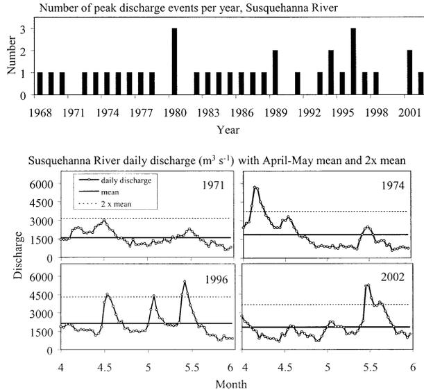
Fig. 2. Number of peak discharge events per year during April and May for Susquehanna River measured at Conowingo Dam. Peak events were defined as spikes in discharge that lasted more than 2 d and exceeded twice the April–May mean discharge. Susquehanna River daily discharge during April and May for selected years (year labeled in upper right corner of each panel). Horizontal lines indicate mean discharge in April and May (thick solid) and twice the mean discharge (thin dashed).
